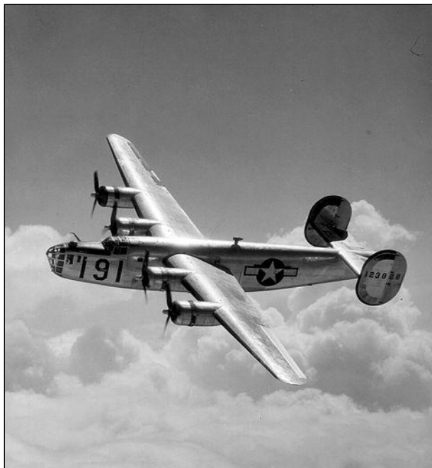
1940: B-24 Liberator: trans-Atlantic capacity (note the slender wings)
