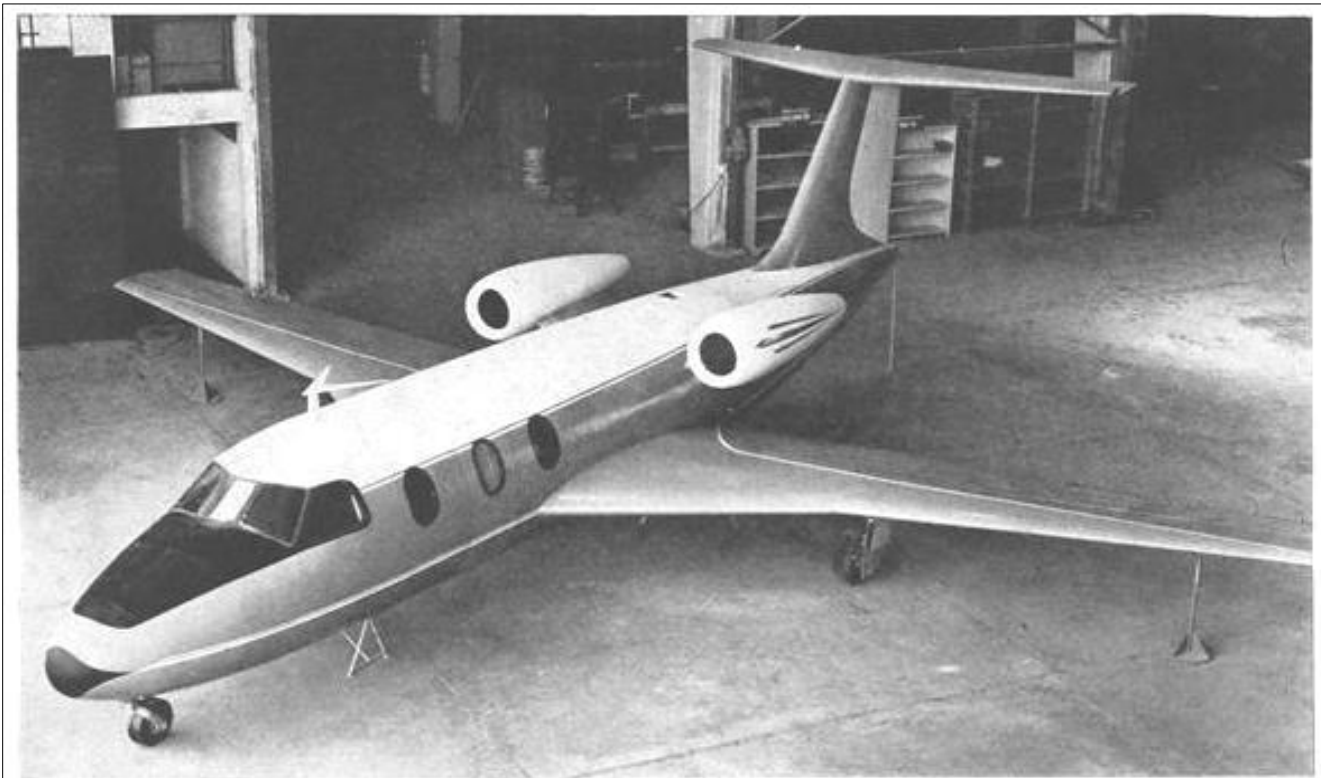
FULL-SCALE MOCKUP of Israeli B-101C executive transport shows T-tail layout of empennage. A V-tail was part of earlier design.
