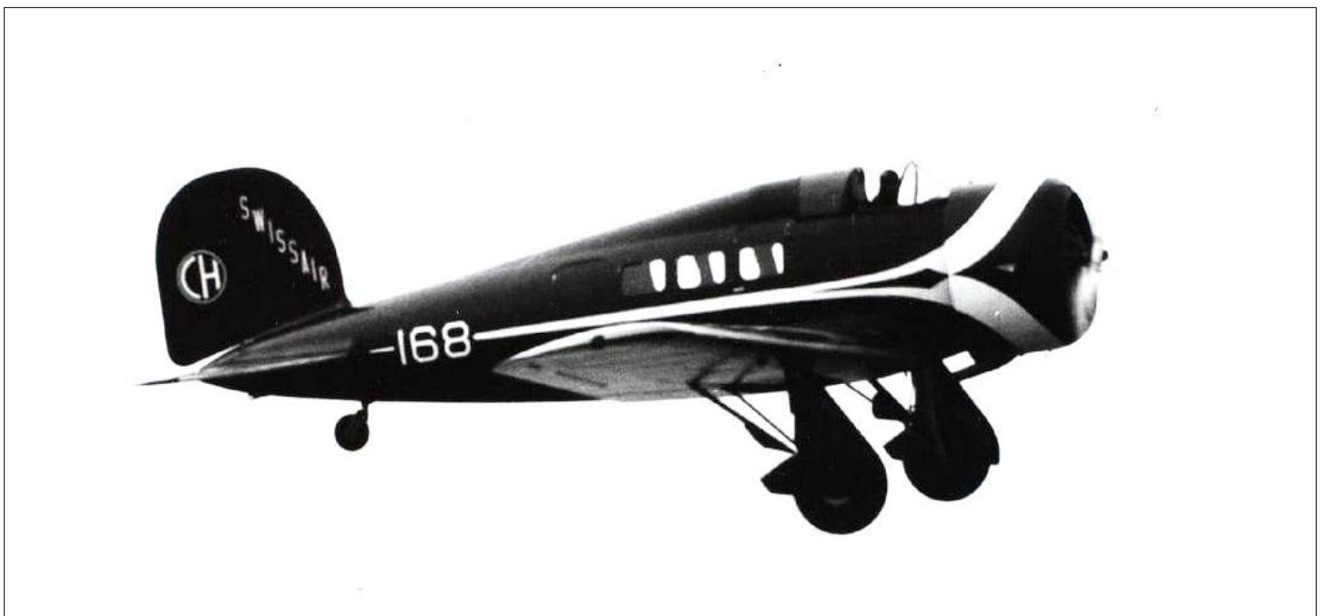
1932 Swissair buys 2 Lockheed Orions, fastest airliner in Europe and the only one with retractable wheels
