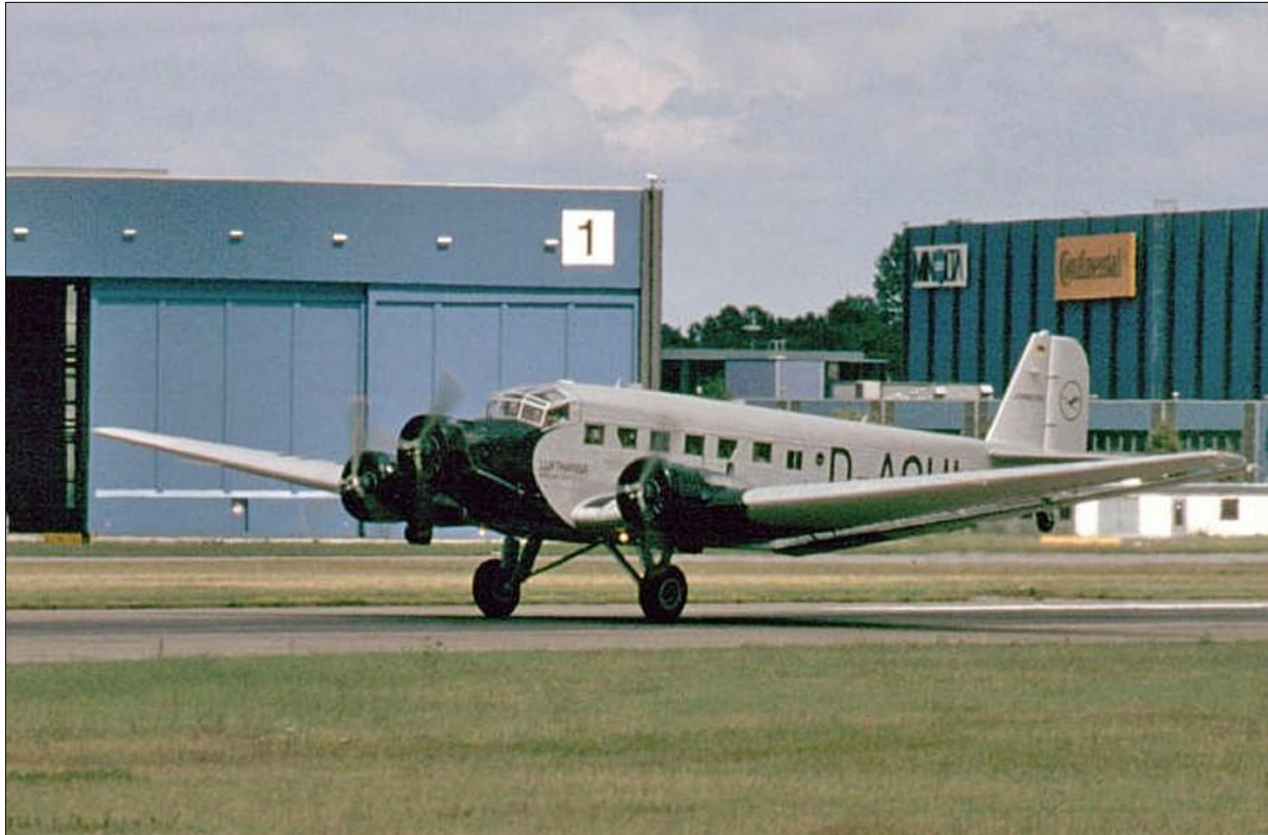
Ju 52-3m, powered by three 550 hp Pratt & Whitney R-1340 Wasp engines. (1932)
