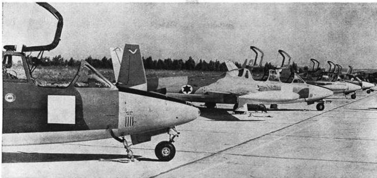
I.A.I.-BUILT POTEZ-FOUGA twin-jet Magister trainers for the Israeli air force are on flight line for final tests before delivery. Operational numbers of the aircraft, already in their military markings, have been deleted by the Israeli censor. Magister is the first aircraft ever to be produced in Israel and is used by the air force as both a trainer and close-support fighter.
