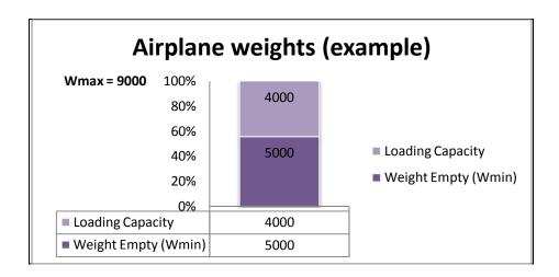
Fig.1 Definition of Weights and Loading Capacity
