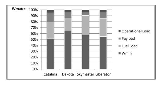
Fig.5a Relative Weights and Fuel Loads for Long Distance Flight (based on Jane's)
