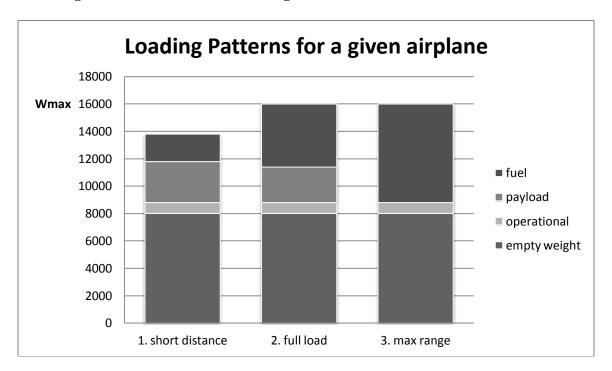
Fig.3 Loading Patterns (example)
