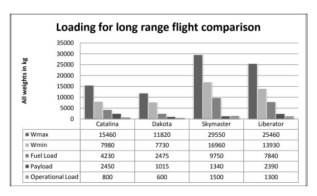
Fig. 5 Weights and Fuel Loads for actual Long Distance Flights (based on Jane's, see Table 3 below)
